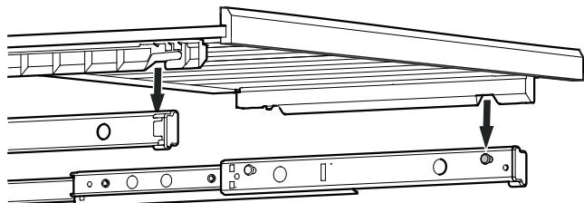
Extend the pull-out rails as far as they will go. Place the front recesses of the wooden shelf on the securing pins.
