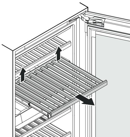
Pull the wooden shelf upwards on the right and left at the back (release) and then remove it towards you.
